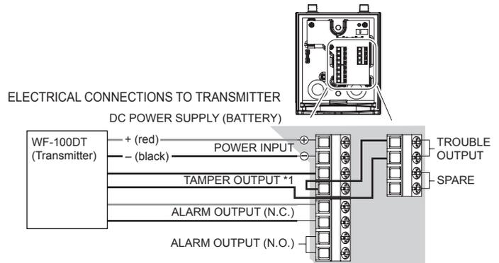
\*1: TAMPER terminals to be connected to a 24 hour supervisory loop.
