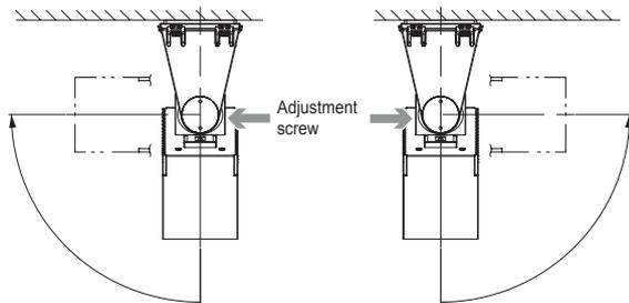
To rotate the unit counterclockwise
