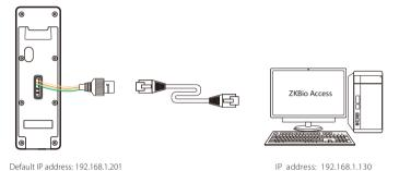
Click on [COMM.] > [Ethernet] > [IP Address], input the IP address and click on [OK].
