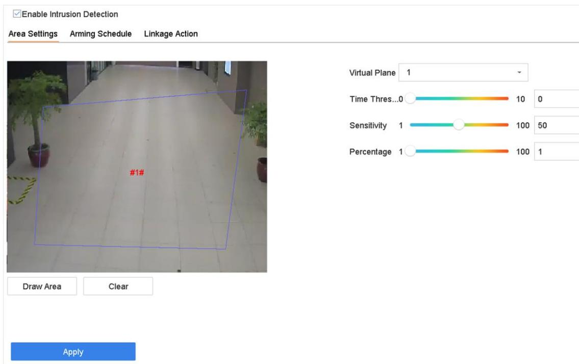
**Figure 5-7 Intrusion Detection**
