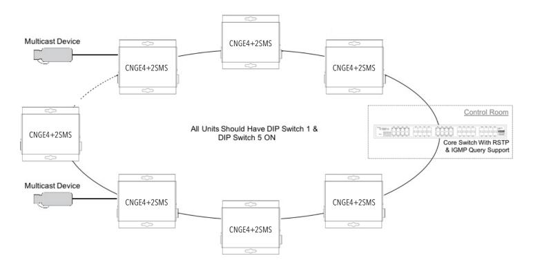
Important Note: The CNGE4+2SMS supports IGMP snooping only. When using the IGMP function a managed switch must be implemented within the network that is configured as the IGMP Querier as shown.
