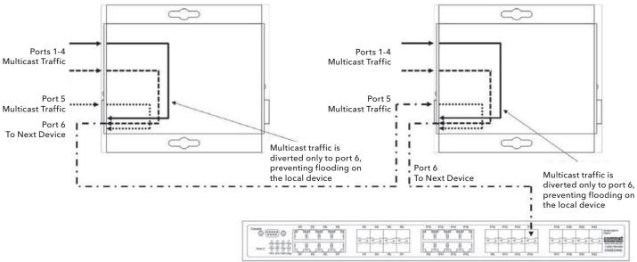
IGMP Enabled on Managed Head End Switch
