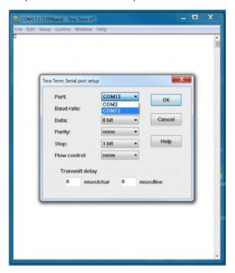
Step 4. The COM port properties setting, 115200 for Bits per second, 8 for Data bits, None for Parity, 1 for Stop bits and none for Flow control.
