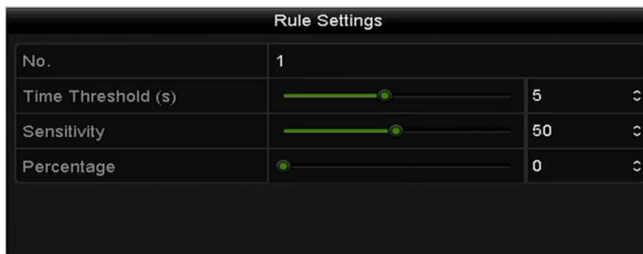
Figure 7-15 Set Intrusion Crossing Detection Rules
