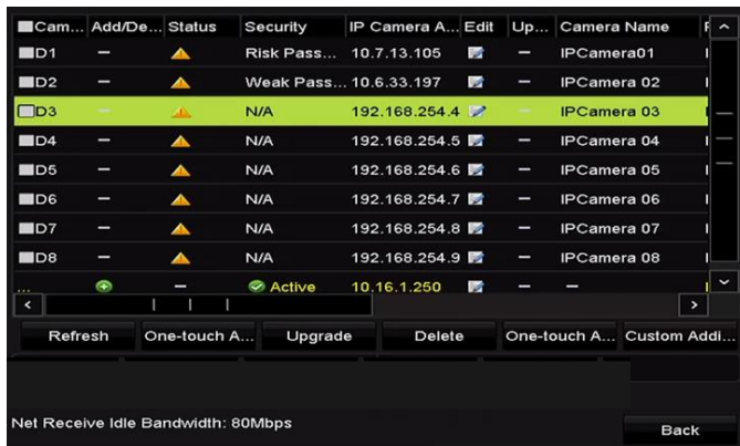
Figure 1-28 List of Connected Cameras
