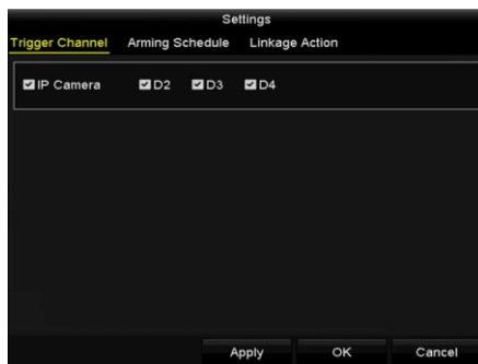
Figure 4-17 Set Trigger Camera of VCA Alarm
