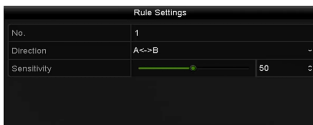
Figure 7-13 Set Line Crossing Detection Rules
