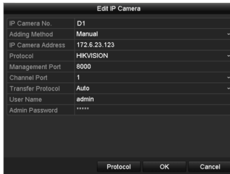
Figure 1-30 Edit IP Camera Interface - Manual
