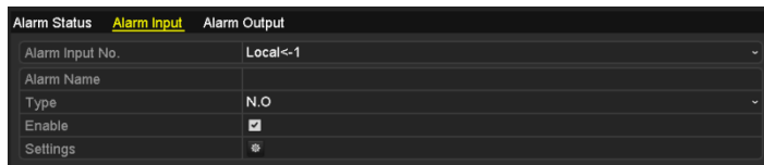
Figure 4-13 Alarm Settings- Alarm Input
