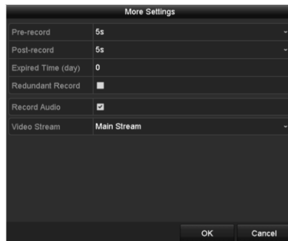
Figure 4-3 Recording Parameters-More Settings
