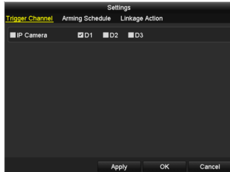
Figure 7-2 Set Trigger Camera of Motion Detection
