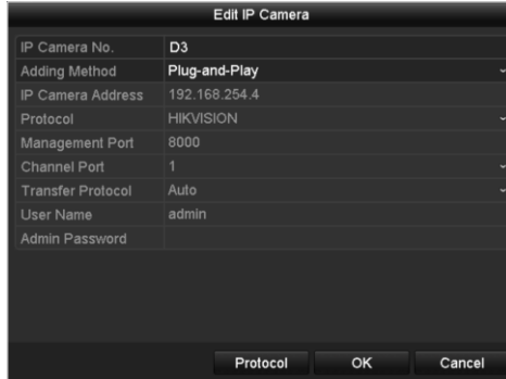
Figure 1-29 Edit IP Camera Interface - Plug-and-Play
