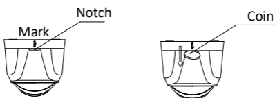
Figure 2-1 Disassemble the Camera
