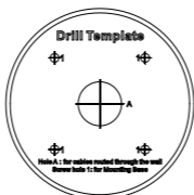
Figure 2-13 Drill Template of the Junction Box
