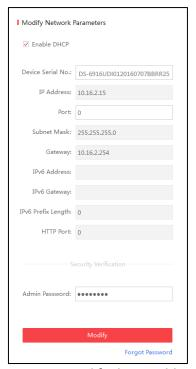
Figure 3-2 Modify the IP Address
