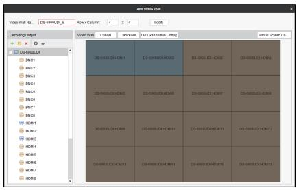
Figure 10-9 Link Decoding Output to Video Wall
