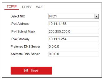
Figure 4-4 Configure Basic Network Settings
