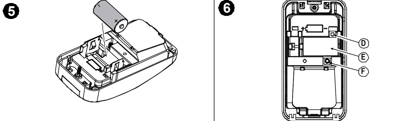
5. Insert battery while observing polarity.
