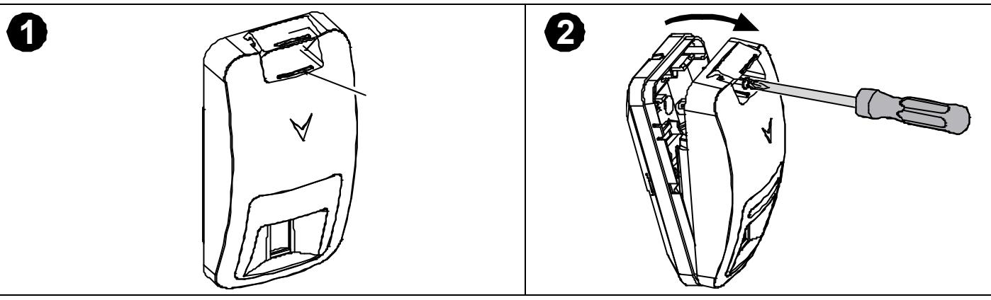
1. On the indicated location, lift the screw cover upward using your thumb.
