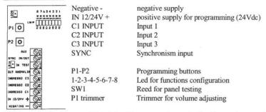
24Vdc panel, with 3 command inputs lauching a pre-set acoustic alert that can be a vocal message or a sound. When more alarm inputs are active at the same time, the last activated one has priority over the others.
