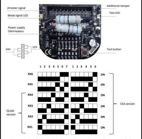
With DIP 7 in ON (as default) and with the power supply LED on, the TX optic functioning is verified. The power supply of the heaters is set by default to 24V; 12V can be used by changing the jumper configuration (SW4) on all optics and on the QUAD B RX board.
