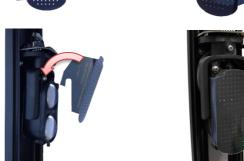
It is sufficient to apply the filter only on the TX, there is no need to repeat the operation also on the  $\mathsf{RX}$ .
