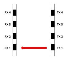
N.B.:During the alignment test phase, the activation of a TX transmitter determines the automatic shutdown of the other TX optics in the column.
