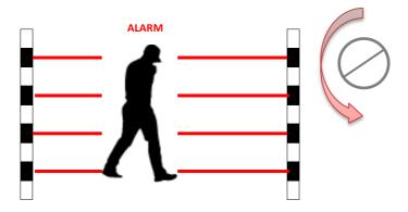
By adjusting the potentiometer anticlockwise, the intervention time is increased up to 500ms.In this condition, the alarm of a person crossing the barrier while walking is guaranteed, with the advantage of excluding the possibility of any false alarms (e.g. animal crossing).
