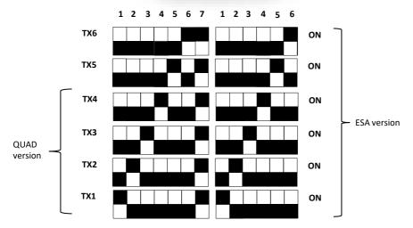
With DIP 7 in ON (as default) and with the power supply LED on, the TX optic functioning is verified. The power supply of the heaters is set by default to 24V; 12V can be used by changing the jumper configuration (SW4) on all optics and on the QUAD B TX board.
