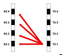
WARNING: too close a distance between the TX and RX columns does not allow calibration with the crossing function.
