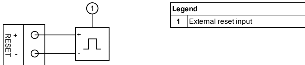
Figure 4-8: Connection for externally resetting the system.
