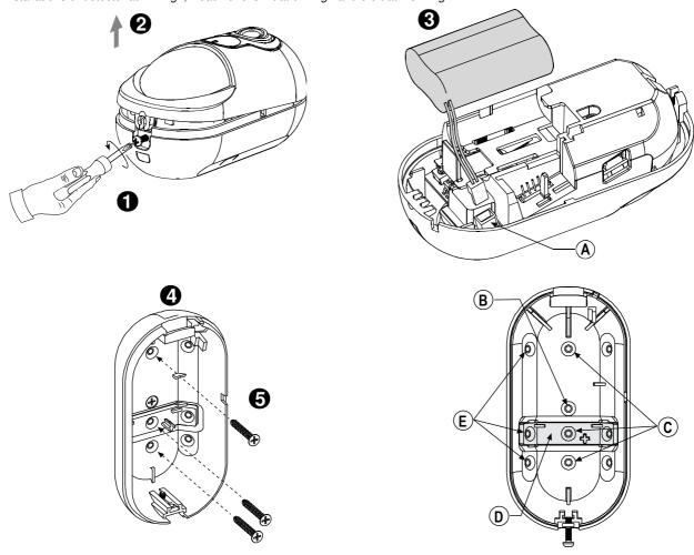
Figure 3a. Mounting on Wall
