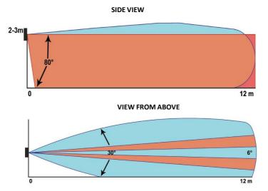
N.B.:The detection zone can vary according to the installation height and the surrounding environment
