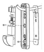
3.After the wiring and the functional test, close the NAT making sure that the gaskets and ORs are present and not deteriorated to guarantee the integrity of the product
