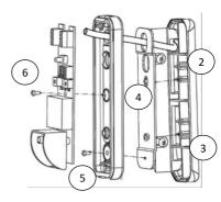
7. After the wiring and the functional test, close the NAT making sure that the gaskets and ORs are present and not deteriorated to guarantee the integrity of the product.
