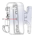
6.After performing the calibration, insert the sensor cover and close everything with the screw located under it
