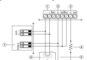
Figure 10: 4-wire smoke and heat detector wiring
