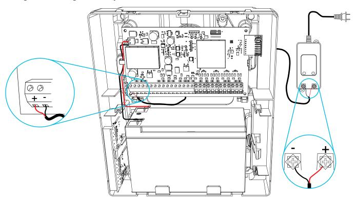
**▶ Important:** You must maintain a minimum separation of 6.4 mm (0.25 in.) at all points between non-power limited battery wiring and all other power limited wiring connections. Do not route any wiring over circuit boards. You must maintain a minimum separation of 25.4 mm (1 in.) between all wiring and the PCB.
