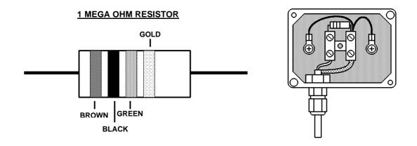
The screen of the sensor cable should be connected into the terminal that is connected to the internal screening of the termination box. This terminal has two black wires connected to it. The termination box can be secured to the fence using the large cable tie supplied or fixed using the mounting holes which are outside the gasket area. Do not drill any holes through the box.
