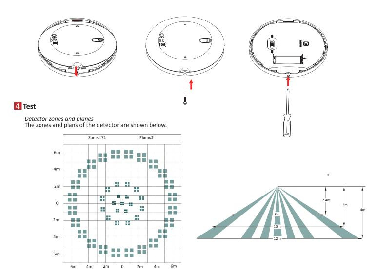
The detector will enter the walk test mode (3 minutes) after being enrolled.
