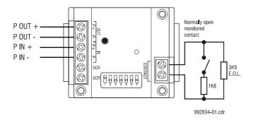
For connection to a Normally Open Contact with wiring monitored as follows:
