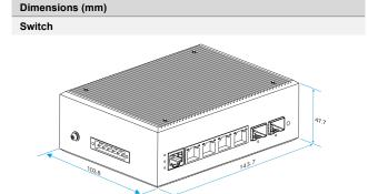
The DIN-rail hanger is fixed on the switch at the factory. Please Install the switch to the DIN rail directly.
