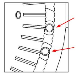
Positioning hole not aligned with slot but positioned at -5°
