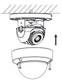
Figure 2-10 Install Bubble
