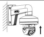
Figure 2-16 Fix the Camera to Wall Mounting Bracket
