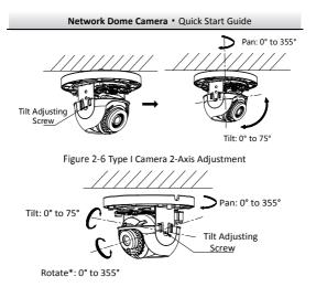
Figure 2-7 Type II Camera 2/3-Axis Adjustment
