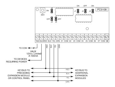
**TAM** - This can be used to tamper the cabinet in which the PC5108 is mounted. Connect a normally closed (NC) switch across TAM and BLK. If the tamper is not being used connect a piece of wire across TAM and BLK to remove the trouble condition.
