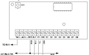
TAM - This can be used to tamper the cabinet the PC5208 is mounted in. Connect a normally closed (NC) switch across TAM and BLK. If the tamper is not being used connect a piece of wire across TAM and BLK to remove the trouble condition.
