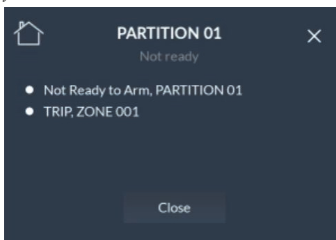
Figure 29: Partition Failed to Arm Screen
