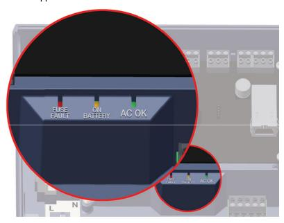
The maximum current that the PSU can guarantee is 1.5A plus 0.5A for battery charging. Beyond this the fuse will trip and the LED will stay on until the load is fully disconnected.
