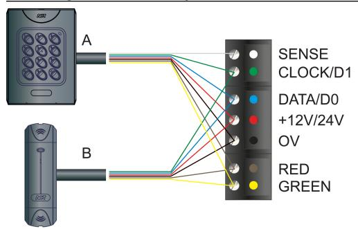
For Clock&Data readers, wire exit readers in parallel with entry readers, but leave the sense line unconnected for exit readers.
