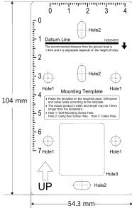
Figure 3-7 Mounting Template
