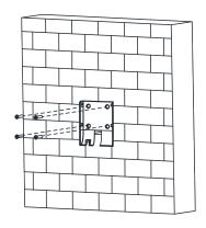
Figure 3-8 Install Mounting Plate
