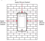
Figure 3-6 Apply Silicone Sealant on the Side
