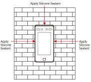
Figure 3-11 Apply Silicone Sealant on the Side
