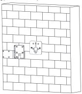
Figure 3-3 Install Mounting Plate
