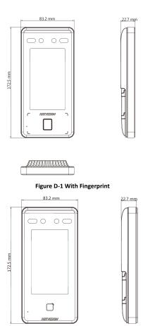
Figure D-2 Without Fingerprint
