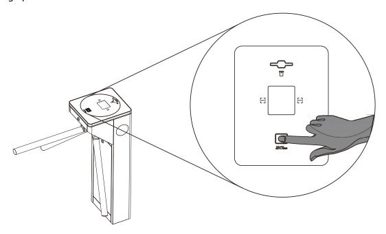
**Recommended fingers:** It is recommended to use index, middle, or ring finger for registration and avoid using the thumb or little finger, as they are difficult to accurately press onto the fingerprint reader.
