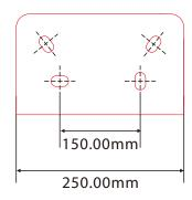
4. Remove the turnstile and use a electric drill to drill holes according to the marks.
