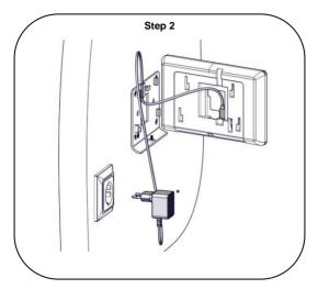
\* 5Vdc/2A Power Supply to USB-C (P/N RP432PSR00A)
