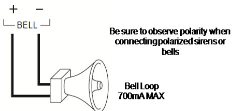
Figure 1-5 Bell Wiring
