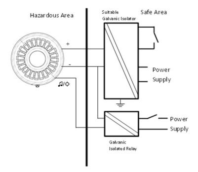
End of line monitoring is applicable to the Sounder Product. For this to function correctly, the resistor must be connected between the IN+ terminal and the Sounder Negative Supply. A suitable Zener Barrier which can allow reverse polarity monitoring to take place and a fire panel compatible with Intrinsically Safe products must also be used.
