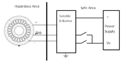
Switching between return paths will enable either Sounder or Beacon, alternately, both the paths could be actived to power both sections together.
