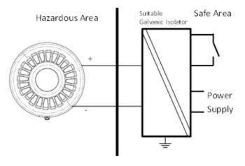
As with the Zener barriers, the Sounder and the Beacon can be triggered independantly when using Galvanic Isolators, however an additional Intrinsically Safe relay is required to make the additional connection.
