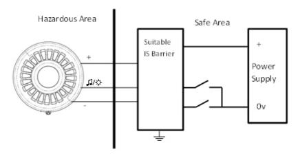
Switching between return paths for the 2 stage system will enable the 2nd tone. Second stage tone can be found in the table on page 12.
