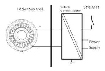
As with the Zener barriers, the second stage alarm can be triggered when using Galvanic Isolators, however an additional Intrinsically Safe relay is required to make the additional connection.
