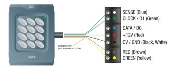
IMPORTANT: To put ACT readers into wiegand mode connect the SENSE on the reader to 0V/GND PIN and DATA/D0 to the SENSE PIN on the controller.
