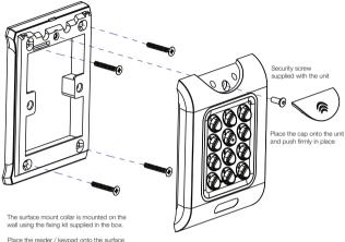
Place the reader / keypad onto the surface mount collar and clip down into place. Use the security screw supplied to attach the unit to the surface mount collar.
