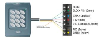
IMPORTANT: To put ACT readers into wiegand mode connect the SENSE on the reader to 0V/GND.
