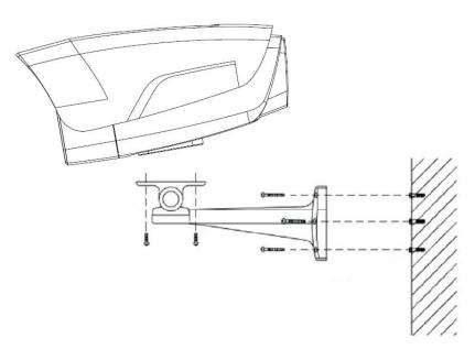
Installation diagram of HD network IR integrated machine
