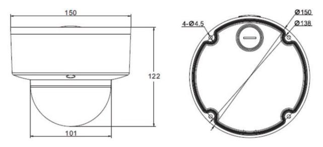
Dimensions of HD Network Zoom (non-)IR Dome Camera - V2.0
