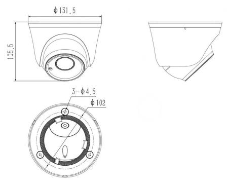
Dimensions of HD Network IR Dome Camera - V3.0
