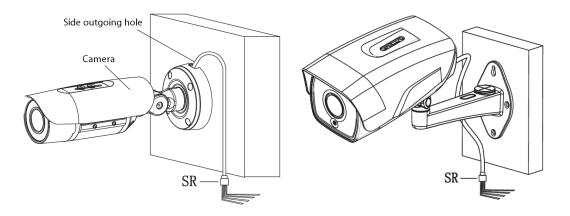
Installation Diagram of Tail Cable
