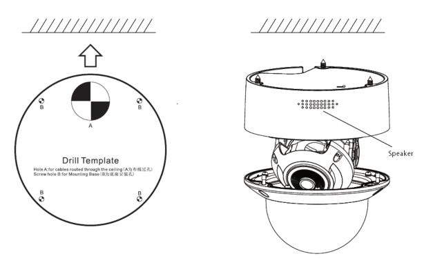
Installation Diagram of HD Network Zoom IR Dome Camera-V3.0
