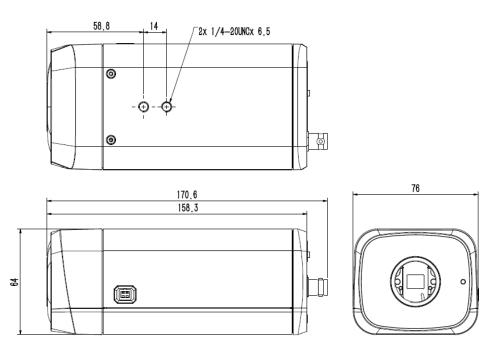
Dimensions of HD Network Gun Camera - V3.0
