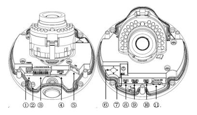
Internal interface of HD network zoom (non-) IR dome camera-V2.0
