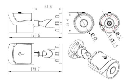
Dimensions of HD Network IR Integrated Machine (MINI)- V1.0
