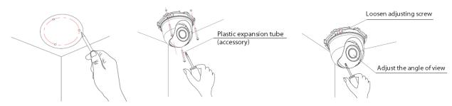
Installation Diagram of HD Network IR Dome Camera (MINI)
