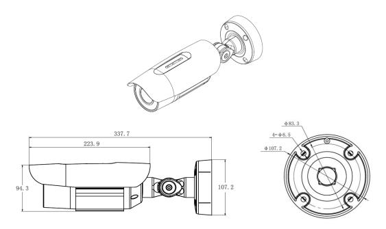
Dimensions of HD Network Zoom IR Gun Camera (with integrated support)
