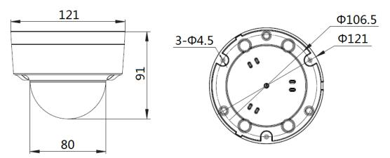
Dimensions of HD Network Safe (Non-) IR Dome Camera - V1.0
