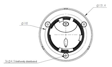
Installation Diagram of HD Network IR Dome Camera-V3.0/V4.0
