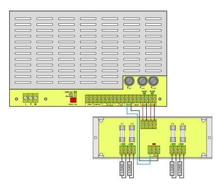
Example of a connection with the fuse module EN54C-LB4.
