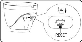
**Note:** For reset (used to return the camera settings to factory default mode), long press for 10 seconds and then the light turns off.
