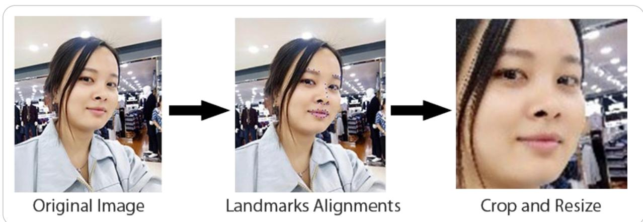
Analyzing the landmarks of input facial image and aligning the image with the pre-saved facial template by cropping and resizing.
