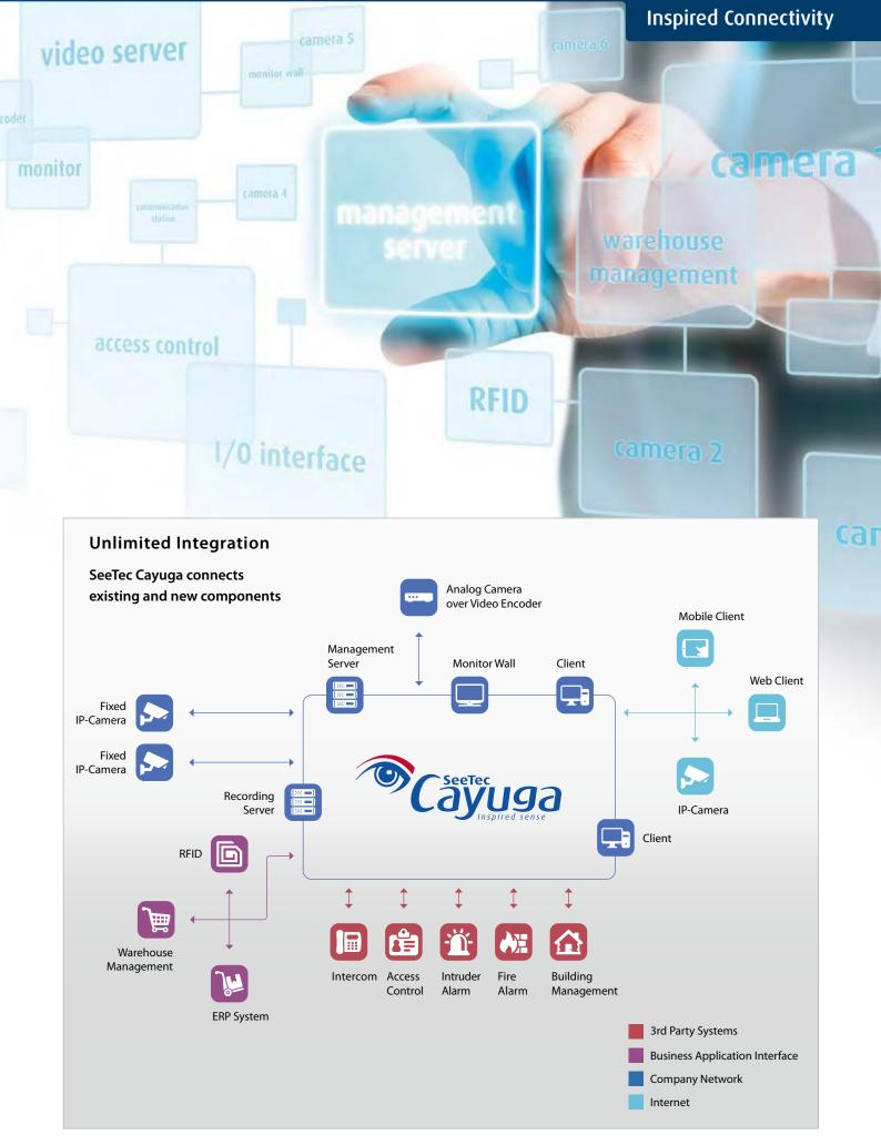
SeeTec Cayuga can integrate a variety of different systems via internet, interfaces, and protocols.
