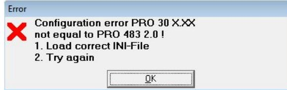
If you do not load any INI-File before selecting a detector, the software will automatically select the correct INI-File for you. If the error message above appears anyway, you're software is not compatible with the detector, please connect our tech support for a software update.
