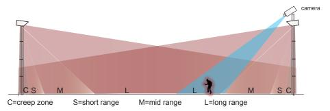
When an intruder appears, PIR alarms are activated and camera streams to ADPRO FastTrace 2E, iFT, CamDisc E or ipVG-Series for visual verification and response by operator.
