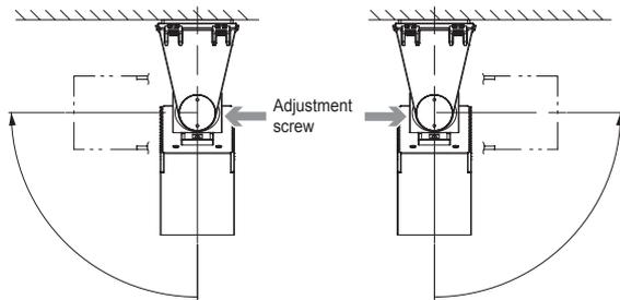
To rotate the unit counterclockwise
