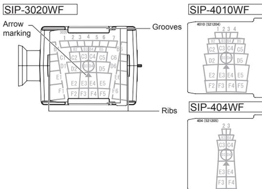
**(5) Fine adjust the main unit angle in vertical and horizontal direction by observing the target area through the area viewfinder.**
