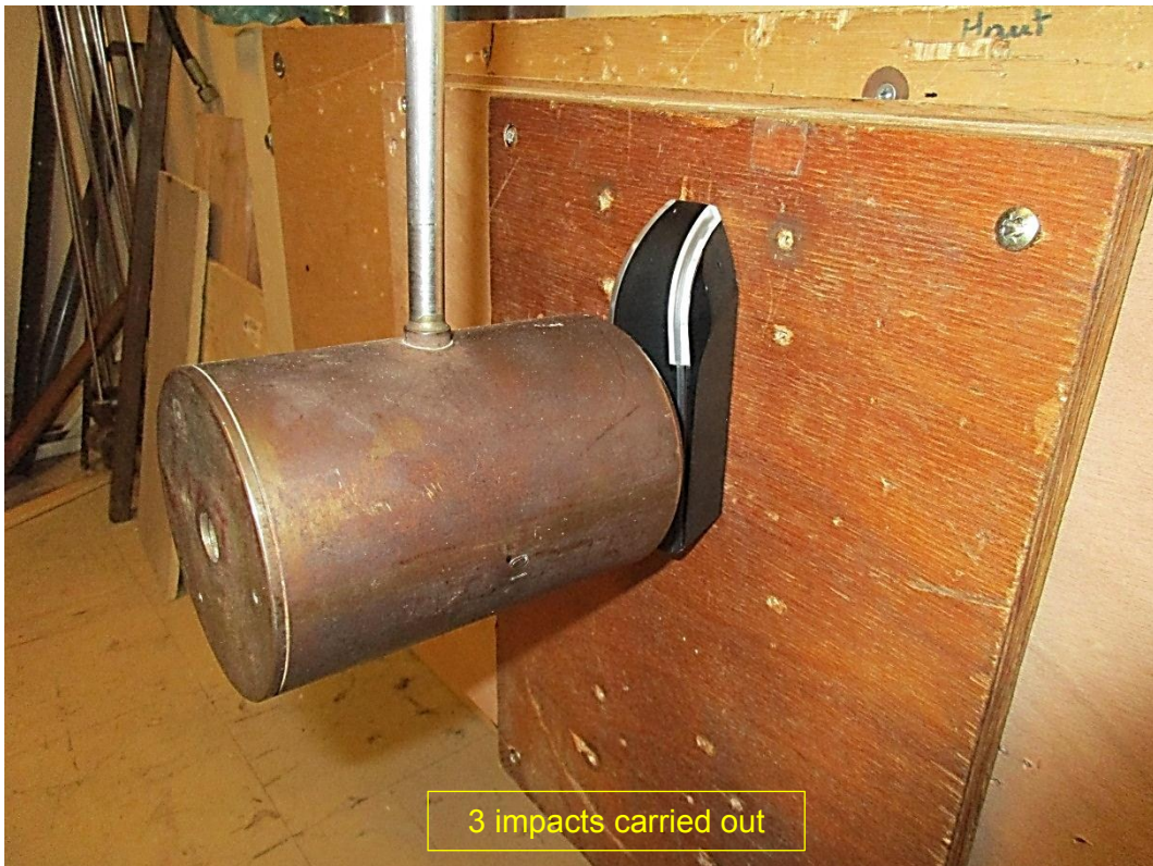
Photograph N°1: Number and location of impacts.
