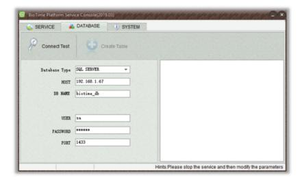
2. If you have not configured the database during installation, you need to select the desired database and enter the correct parameters then click **Connect Test**. It will display "Connected Successfully" if the connection was made successfully.
