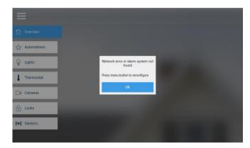
On the first startup, you will see a network error message because the touchscreen is not connected to a Wi Fi network. Press OK. Press the menu button to configure the touchscreen. The touchscreen will ask you for a PIN.
