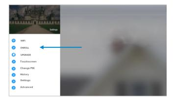
The touchscreen will automatically find any available hubs on the network. They appear in the left column. Select the desired hub from the network displayed. Enter the installer PIN that is set up for the hub.
