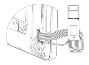
Connect a high gain antenna to the antenna socket shown below and retest signal level.
