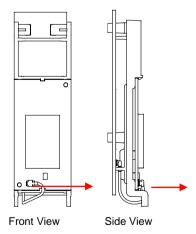
Gently push retaining clips outwards and remove rear circuit board. This is the internal antenna which will no longer be needed.
